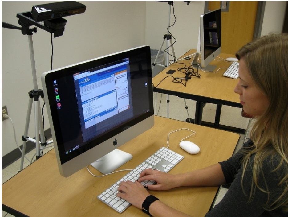
Figure 2: Multimodal instrumented tutoring session, including a Kinect depth camera to detect posture and gesture, a webcam to detect facial expression changes, and a skin conductance bracelet to detect electrodermal activity.
