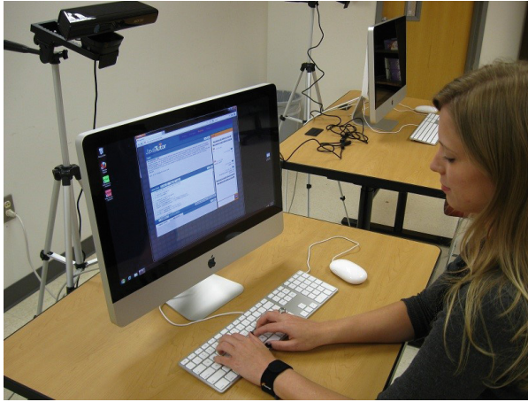
Fig. 2. Multimodal instrumented tutoring session, including a Kinect depth camera to detect posture and gesture, a webcam to detect facial expression changes, and a skin conductance bracelet to detect electrodermal activity.
